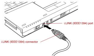
Figure 3-29 Connecting the i.LINK (IEEE1394) cable into the computer
